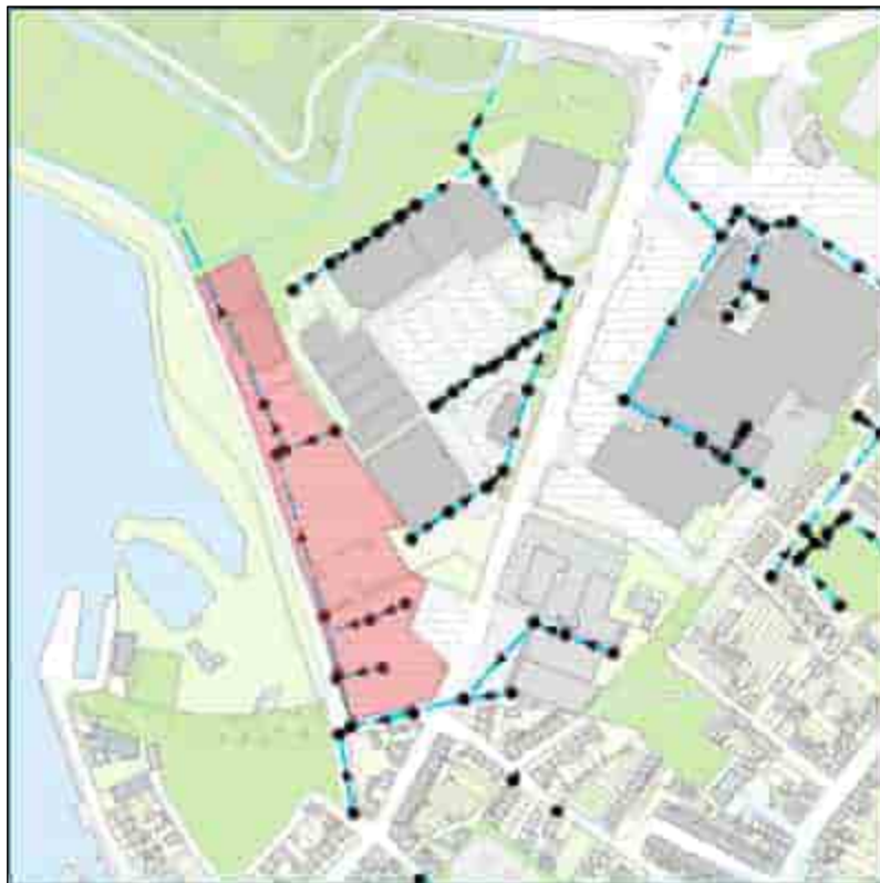
Figure 2-1: Existing Surface Water Infrastructure, UÉ 2024
